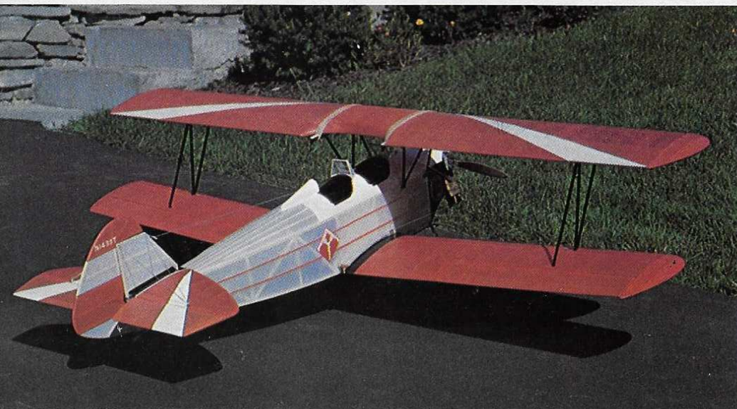
You can always tell a Fleet—most of them anyway, because there were some early Army primary trainers—by that characteristic rudder with so much area down around the fuselage center line.
