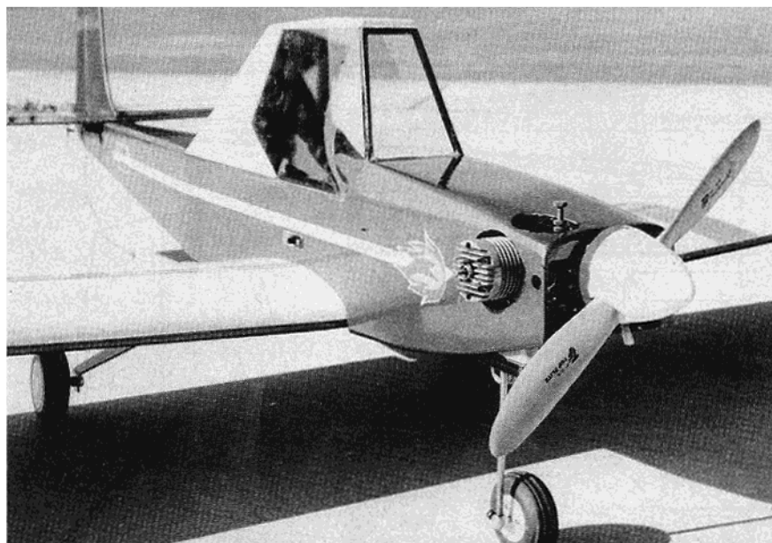
Bottom view of engine compartment. Nose gear leg goes through engine mount. Bottom could be closed in.
