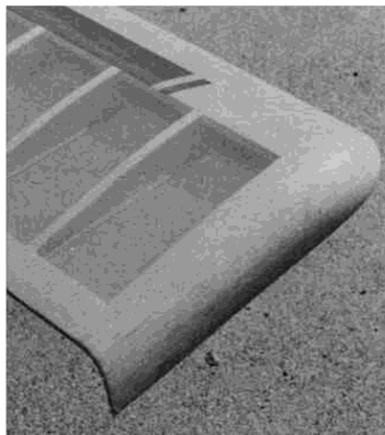
Hoerner vortex tip is not difficult to carve and provides that extra touch. You can inset 1/16 wire for extra strength.
