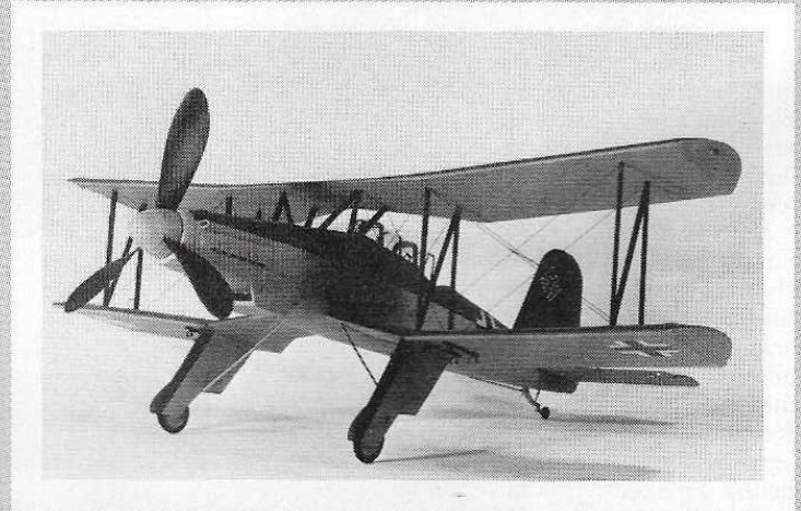
Covering is white tissue, conventionally applied, and finished with water thinned Polly S paints after applying two coats of thinned dope.
