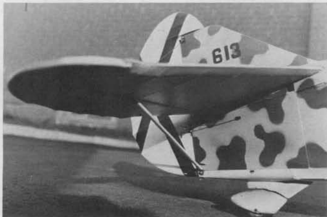
Rudder control and tailwheel detail of the Fiat.
