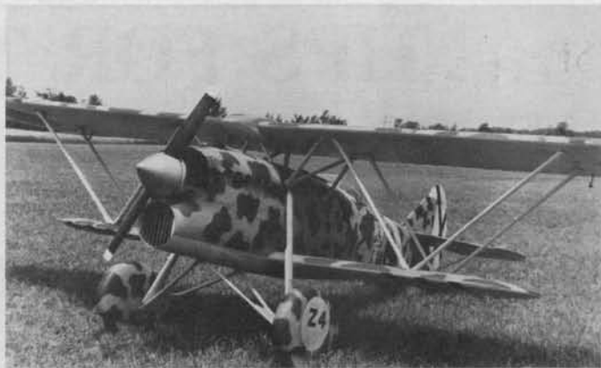
The CR 32 ready for a flight. Total weight of the author's model was 10-1/2 pounds. This plane has made 80 successful flights to date.
