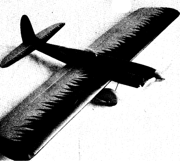
With the larger wing and inverted engine, slowed-down Fenó proved ideal for the special flying conditions the designer had to contend with.
