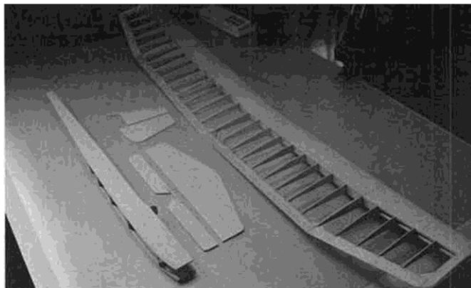
The bare bones of the Feather before final assembly and covering. There aren't more construction photos because construction is so darn easy! Anyone with some building experience can do the job.
