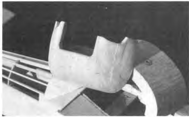
Front view of lower cowl with hatch in rear.
