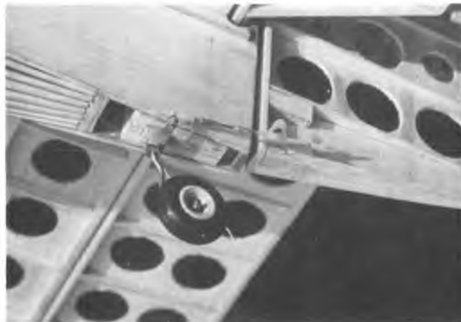
Close-up of tail wheel and linkage detail.
