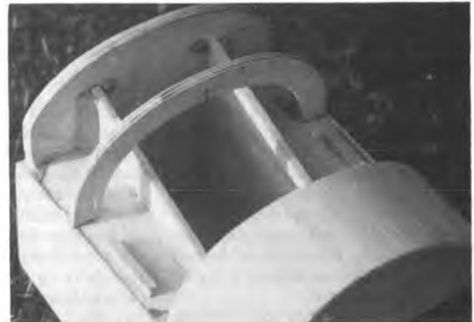
Top front of fuselage with hatch and cowl removed.
