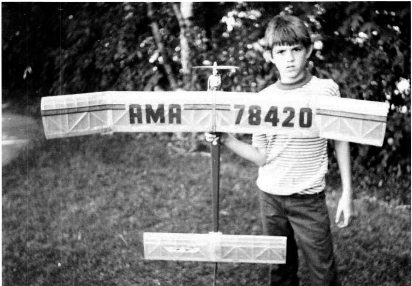
Bob Stalick's son, Ted, above, built the FAIMan 7 shown in these photos. Ship is relatively small as FAI power models go, but is not any less capable of doing the job. Could also be built for 1/2A-A power, but would be mild with the thick airfoil shown.
