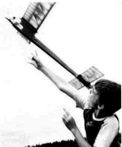
Up, up, and away! Model climbs in right spiral and makes about two turns in a 10 second run.
