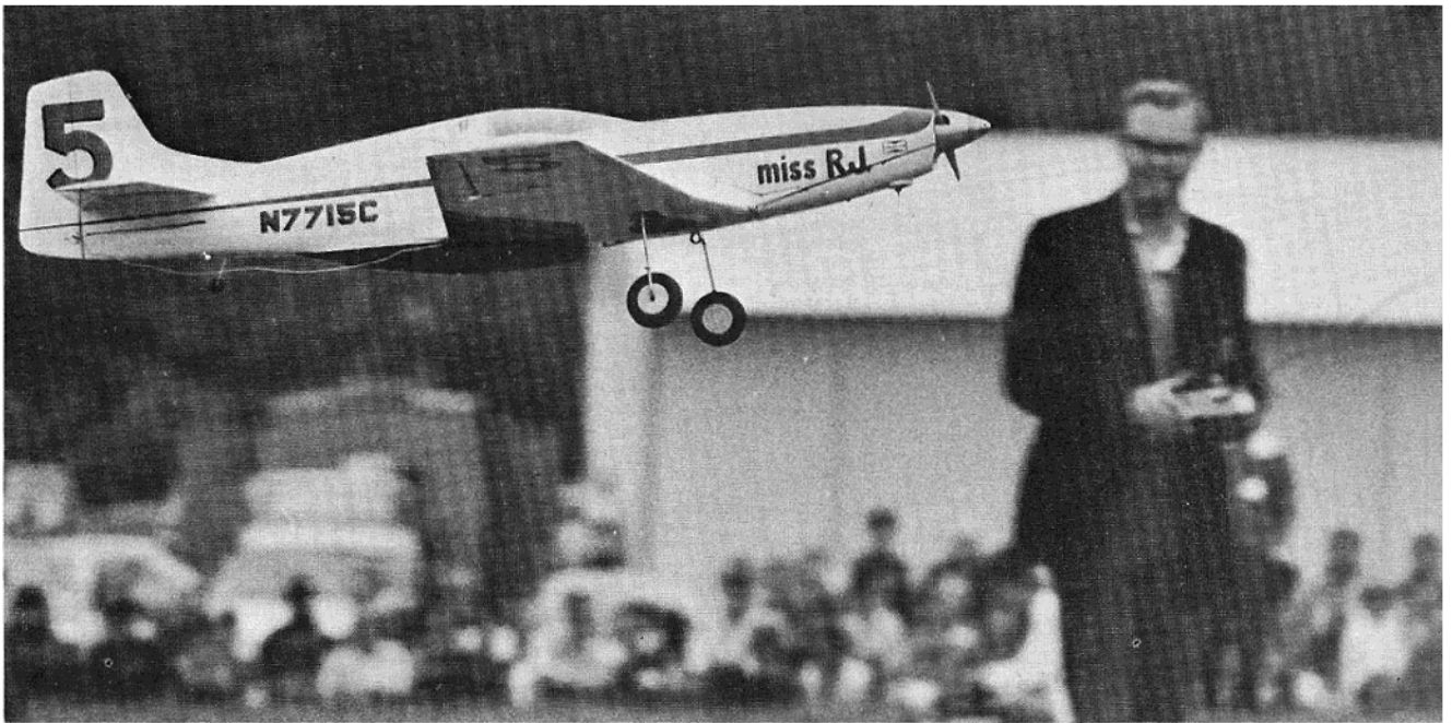
Prototype No. 2 follows lines of Chuck Hall's "Miss R.J." Had fixed gear, Lee Custom K & B .40. Eric Wall holds model ready for takeoff at right. Above, a dead stick landing.
