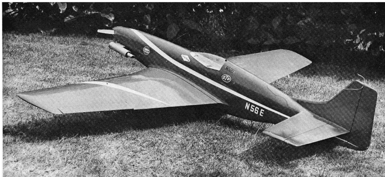
Mustang F.A.I. built by John Evans of Scarborough, England, features K.D.H. Mini retract gear. Kraft radio, K & B .40 with KO muffler.
