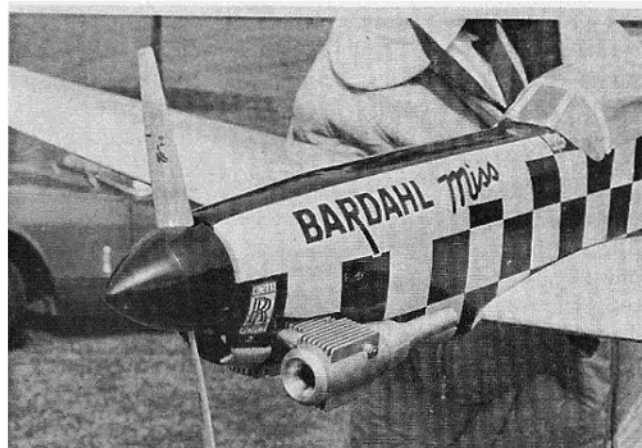
Nose close-up showing Super Tigre S.56 air scavenged type muffler. Large muffler right behind engine creates much drag. Next step is to incorporate muffler within cowl. Reworked T/F 9 x 8 prop shown - T/F 9 x 7 Speed prop., cut to 8 3/4" worked best with K & B .40. "Bardahl Miss" decals available from designer on request, also "Miss R.J."
