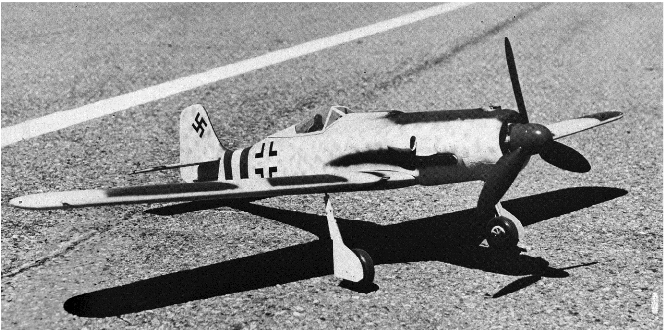
The Ta 152's stretched span, additional effective dihedral and increased washout make the model a very stable flyer.
