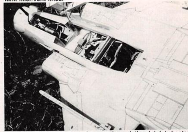
Flap and aileron servos can be seen through the air inlet cheater hole. Extensive panel lines add much to overall finish. Also, note location of air control valve for retracts.
