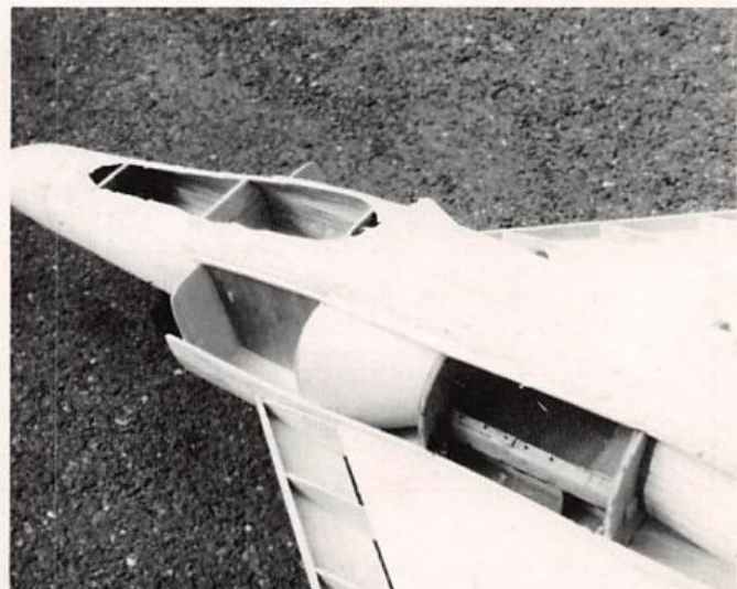
The actual shape of the ducting cannot be shown on the plans, so it must be made via the cut and fit method. Be sure to get good glue joints at all contact locations.
