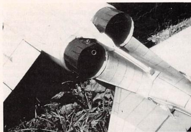
Jet outlets made up from stiff paper or 1/64" plywood. 1/32" ply strips form "eyelets" and are glued to outlets.
