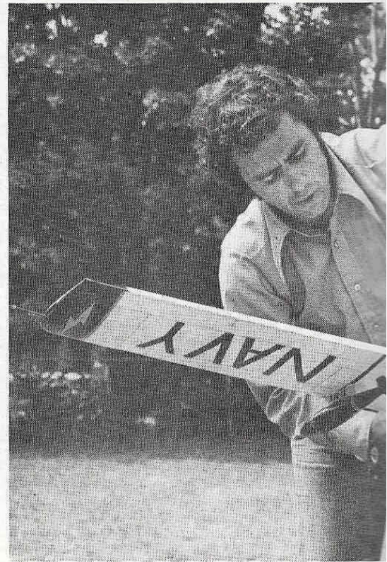
How a model hangs out on the lines is half the battle. Adjustable leadout permits on-field adjustment of line rake. Easy to install, quick to set. At right: Vic has his hands full. It's a fair sized machine, all the area you'll need for cornering, pattern aerobatics. Use a good .35 powerplant.
