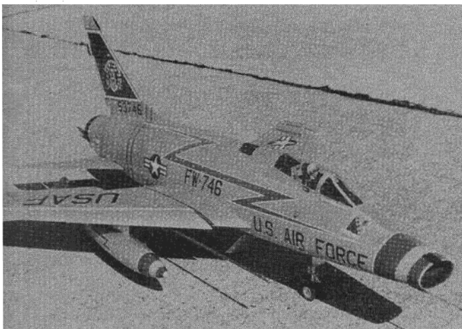
Leading edge slats on the original floated and were positioned by air pressure. On the model they are positionable, here shown fixed in take-off and landing position.
