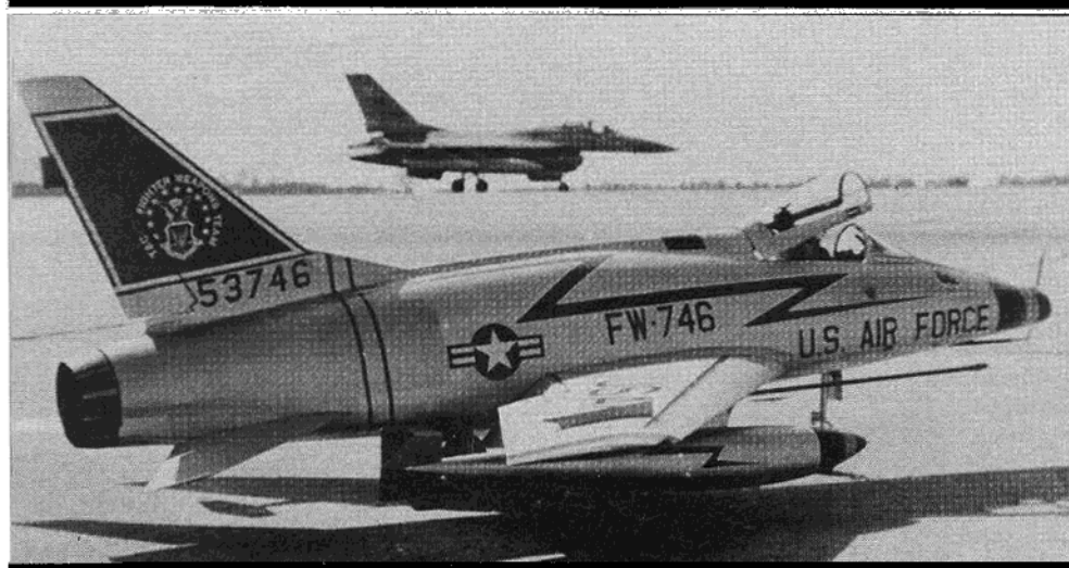
Below; Sequence photos of the F-100D on a fly-by pass. It looks like the real thing from any direction. Flight trim position of full flying stab is readily visible.
