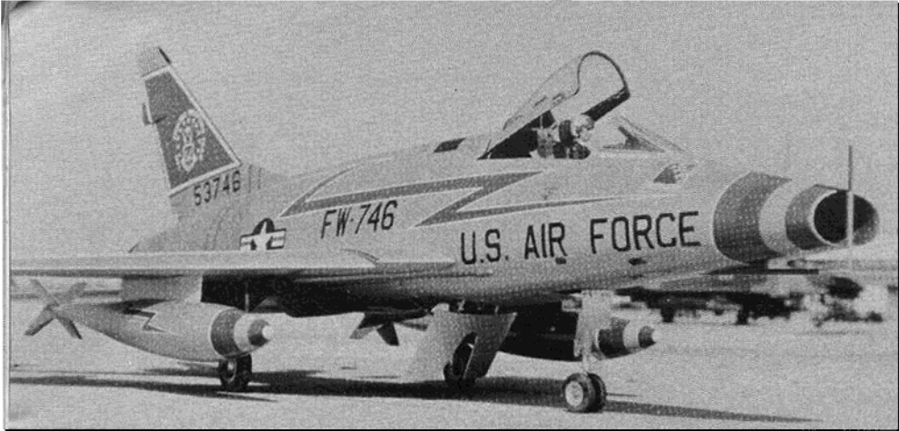
Art Johnson's F-100D on the ramp at Eglin AFB, Florida. The model is painted as it was when Art flew it in the first world wide All Supersonic Fighter Weapons Championships at Nellis AFB, Las Vegas in 1958. (See color shot on previous pages.) The 12.5 pound model is a little less than 1/8 scale and is powered by a Rossi .81 turning a Byron fan.
