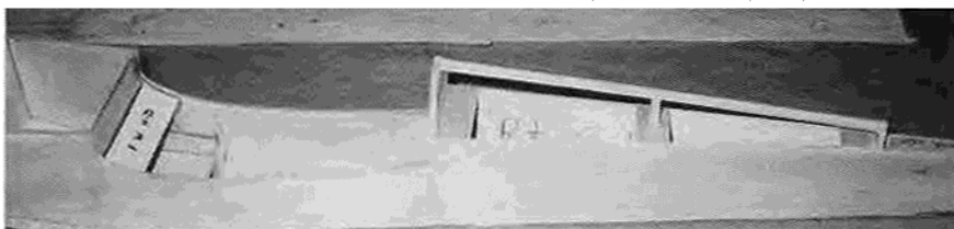
After bottom is sheeted, turn right side up and add turtledeck formers, stringer, and wing hold-down blocks.
