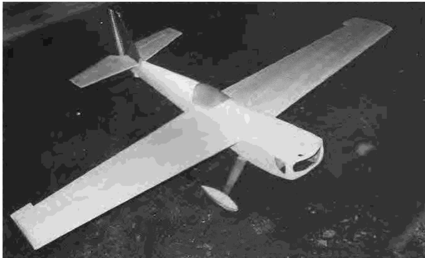
Completed airframe sanded and ready to cover. Vertical fin was salvaged from Prototype #1.
