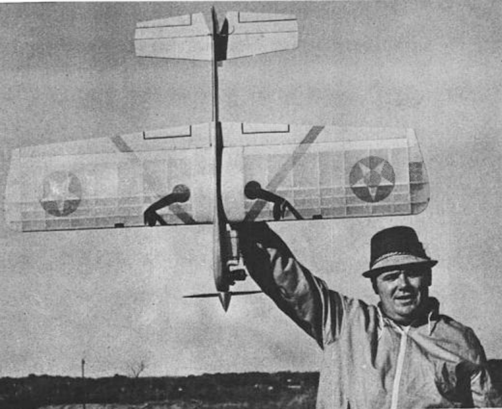
Wide landing gears make for smooth landings, add to realism, tough. Note black tissue gums and landing lights on leading edge.
