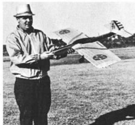
Low drag is important for good flying, and you can see how this can be done on a profile design, still maintaining realism.
