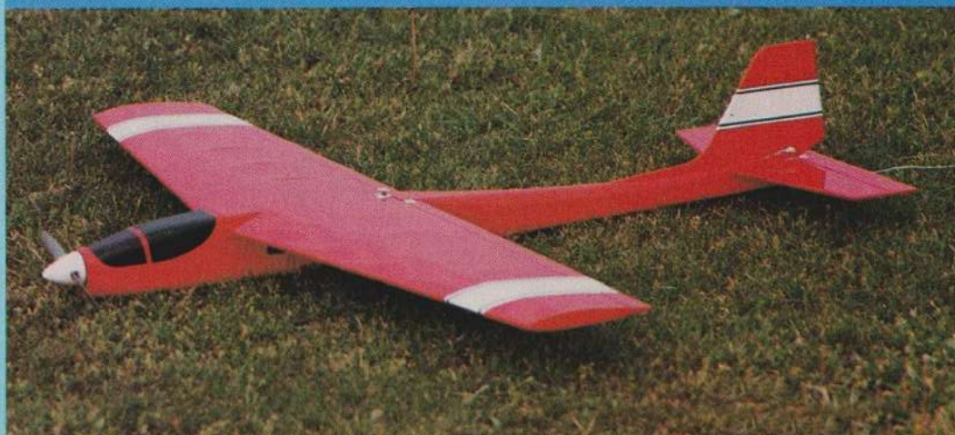
Top: The basically all-red color scheme is simple, light, and shows up well in the air. A little white and black trim on the upper surface helps to tell which side is which during aerobatics. Above: A flyby shows the sleek lines of the Electrostream. The long tail moment provides excellent stability, yet surprisingly allows a crisp snap-roll and spin with immediate recovery. Below: Tom's model has been mistaken for a slope soarer; it might make a good one at that.
