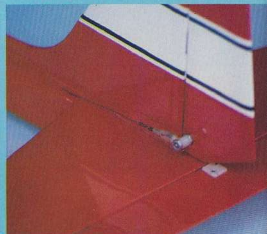
The rudder is controlled using a pull-pull cable system made of nylon-coated steel leader line. This setup is very solid and extremely light. Perfect for an Electric model.
