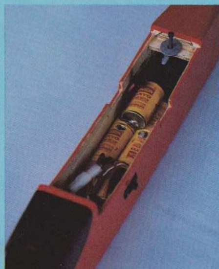
A crowded radio compartment is the sacrifice for a sleek, good-performing aircraft. Just behind the seven-cell hump-style battery pack are the elevator and rudder servos.
