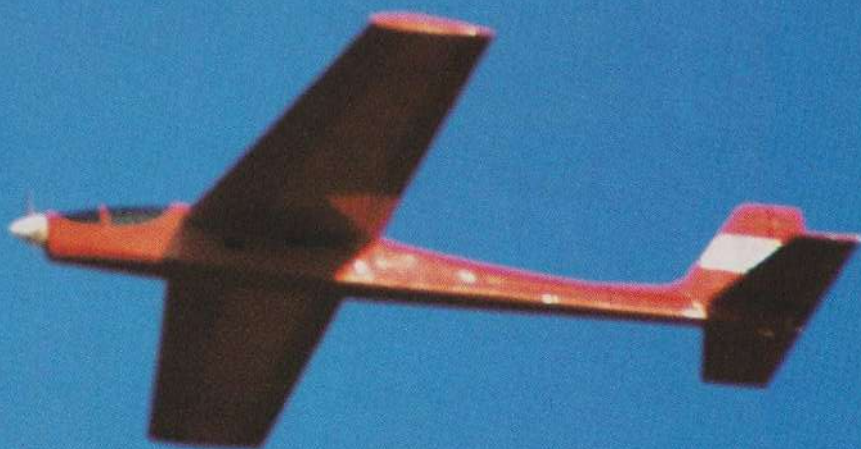
Top: The basically all-red color scheme is simple, light, and shows up well in the air. A little white and black trim on the upper surface helps to tell which side is which during aerobatics. Above: A flyby shows the sleek lines of the Electrostream. The long tail moment provides excellent stability, yet surprisingly allows a crisp snap-roll and spin with immediate recovery. Below: Tom's model has been mistaken for a slope soarer; it might make a good one at that.
