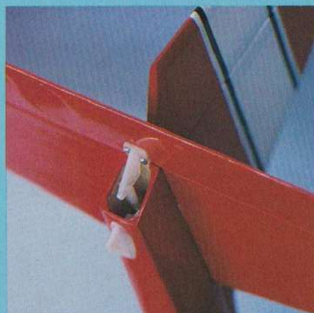
At the tail end is the combination air/pushrod/antenna exit hole. The tail skid is not necessary, being left over from an unsatisfactory attempt to add landing gear, which turned out to be more drag than it was worth.
