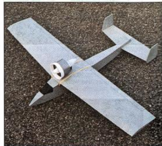
The prototype Electro-Screamer by designer Don Belfort. Simply mounting the fan unit above the wing avoids the complexities and hassles of an internally mounted installation. Wing could easily be bolted on if you're not partial to rubber bands.
