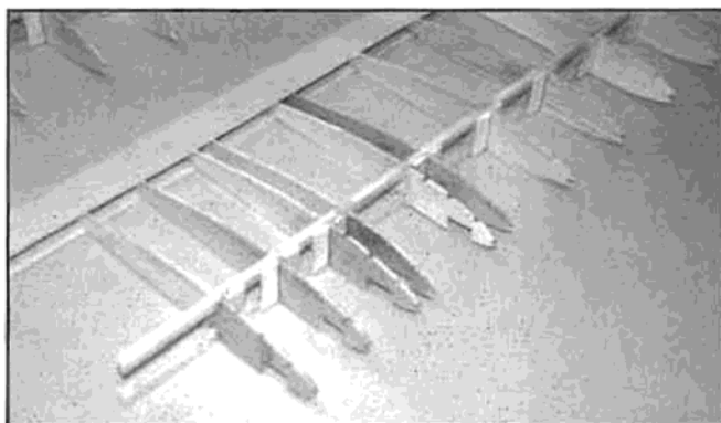
LEFT: Wing assembly under construction. Note the 1/32" plywood doublers attached to ribs for landing gear mounts and spar braces/shear webs glued in place. RIGHT: Assembling the nacelles to the wing. Thread the L.E. dowel and 1/8" sq. turbulator spars through the N1 nacelle sides.
