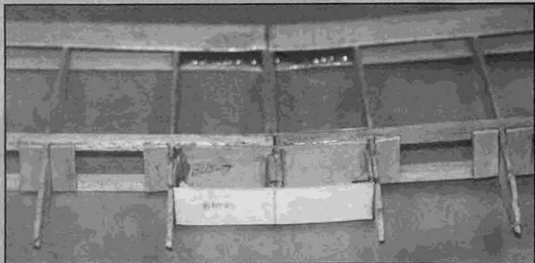
LEFT: Center section trailing edge is filled in to provide anti-crush for wing bolts. RIGHT: Top view of bottom wing with strut braces in place. 1/16" balsa sheet is to aid in covering.
