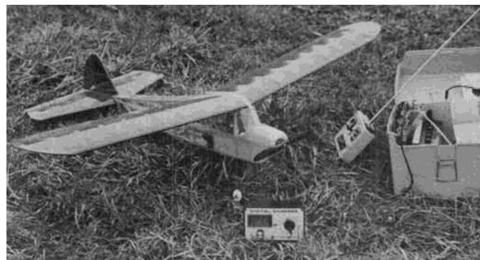
Brigadier gets "refueled" through Leisure Electronics digital charger, from large battery in field box.
