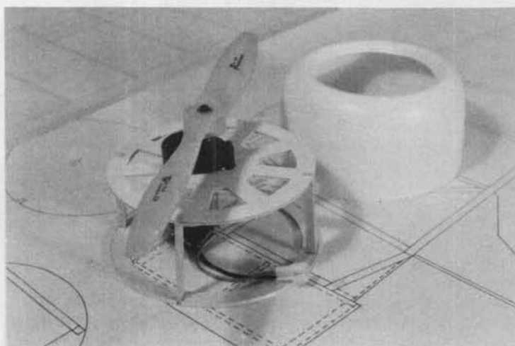
The inside structure of the cowl, and the motor mount. Cooling holes are necessary for the electric motor, and to simulate radial engine.
