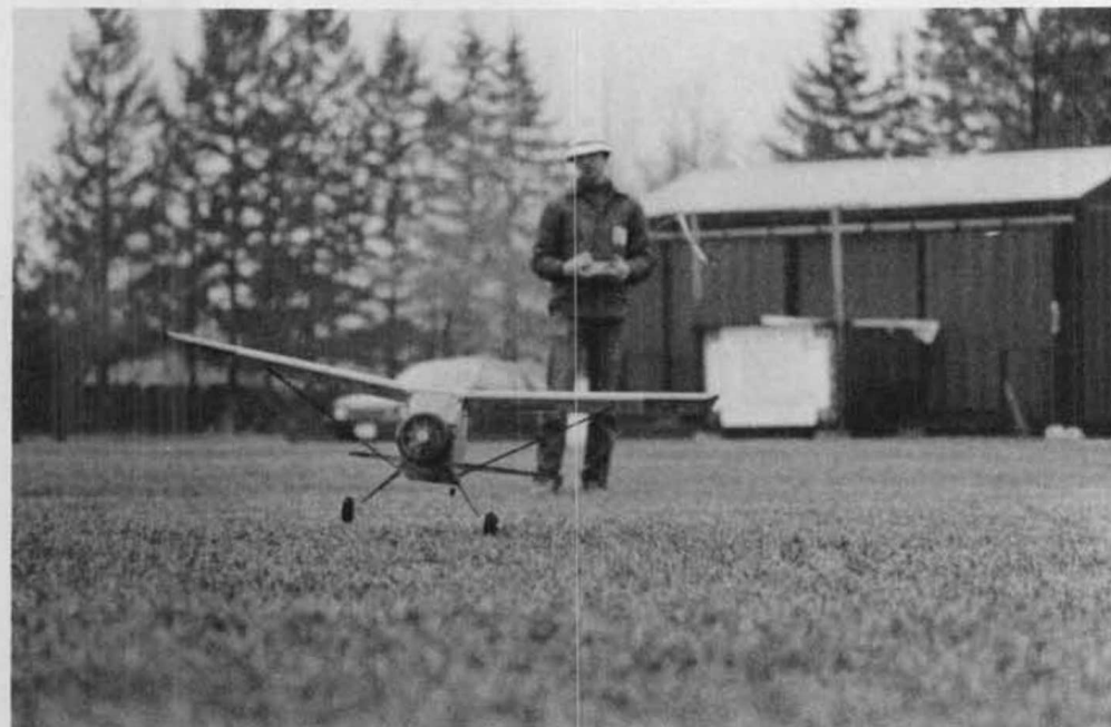
The author's Beaver, eagerly heading for the cameraman, comes in at 48 ounces. Power is from a Leisure gear drive O5 system, with a six-cell 1200 mah Sanyo battery pack.
