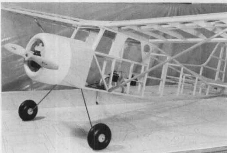
Completely framed and with radio and motor installed, the Electric Beaver is a pleasing-looking little model.
