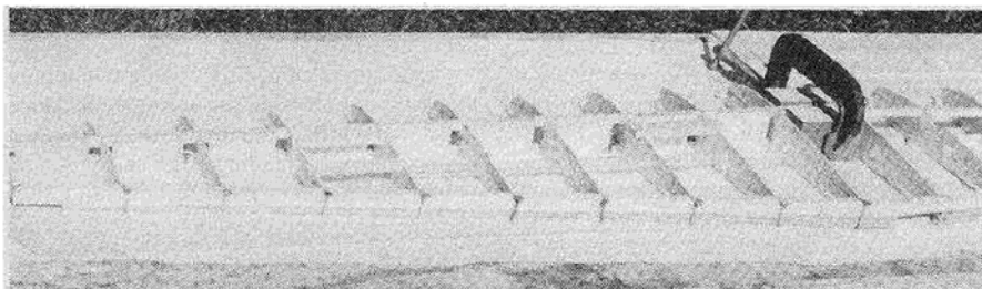
Epoxying and clamping of the main spar doublers.
