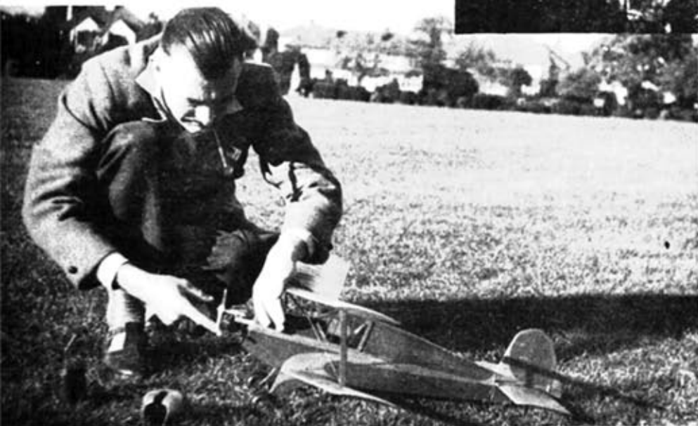
Fly without a cowl, too, says George cranking up his Mac .049 Diesel. Plenty of mills to use.
