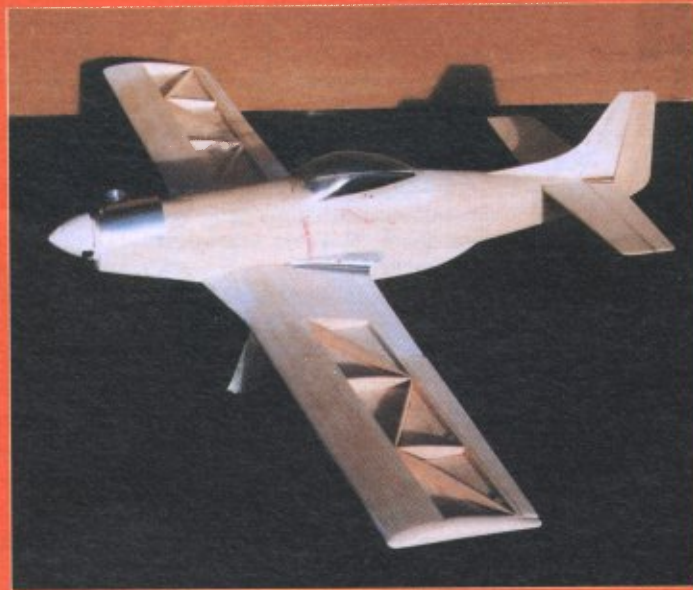
The P-50+1 follows the author's basic EEE-Z-FLL design philosophy: flat bottom wing with fully sheeted undersides and partially sheeted top, and sheet balsa fuselage and tail surfaces. Cowl top, wing root fairings and landing gear fairings are bent from soft sheet aluminum. O.S. 25FP used on original.
