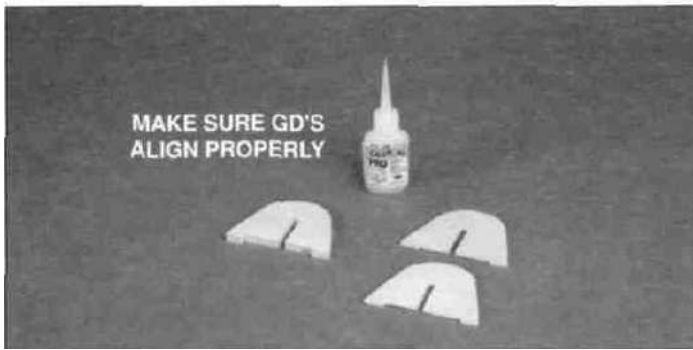
D 3. Locate the four landing gear doublers (GD) and glue together in pairs using medium CA as shown. Make sure that the slots in the landing gear doublers align.
