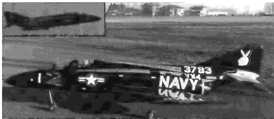
Photo #1: An F-4 Phantom "Black Bunny" scratch-built by the authors with Byrojet fan unit and Rossi 81 engine.
