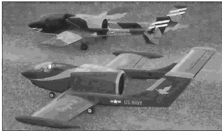
Photo #7: The ducted fan Eagle I (behind) and the Eagle II. A featured construction article ten years ago in RCM (plan #1159).
