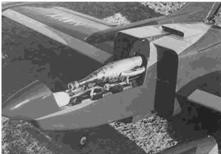
With the canopy/hatch removed, you can see the retract air bottle, radio equipment, tuned pipe, etc.
