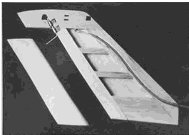
LEFT: Right fin before covering, seen from the outside. Note the elevator flexible control cable. RIGHT: Assembling the left fin to the stab, before bottom sheeting is added.
