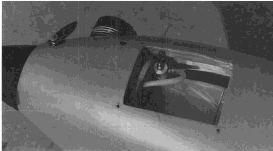
Tank compartment holds 12-oz. Sullivan tank and canister-type filter. Tank is wrapped in plastic to prevent fuel from getting to the radio battery underneath, in the case of an unnoticed leak.
