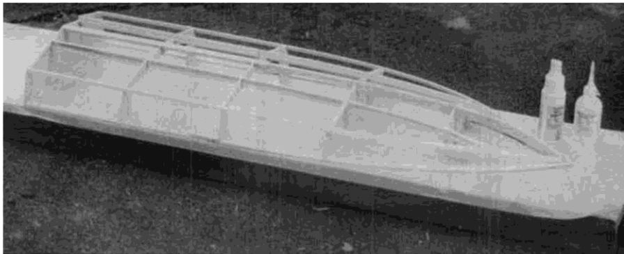
Hull framework is built on FLAT building surface. Hot Stuff Super T and Hot Shot Accelerator were used to speed up the building process.
