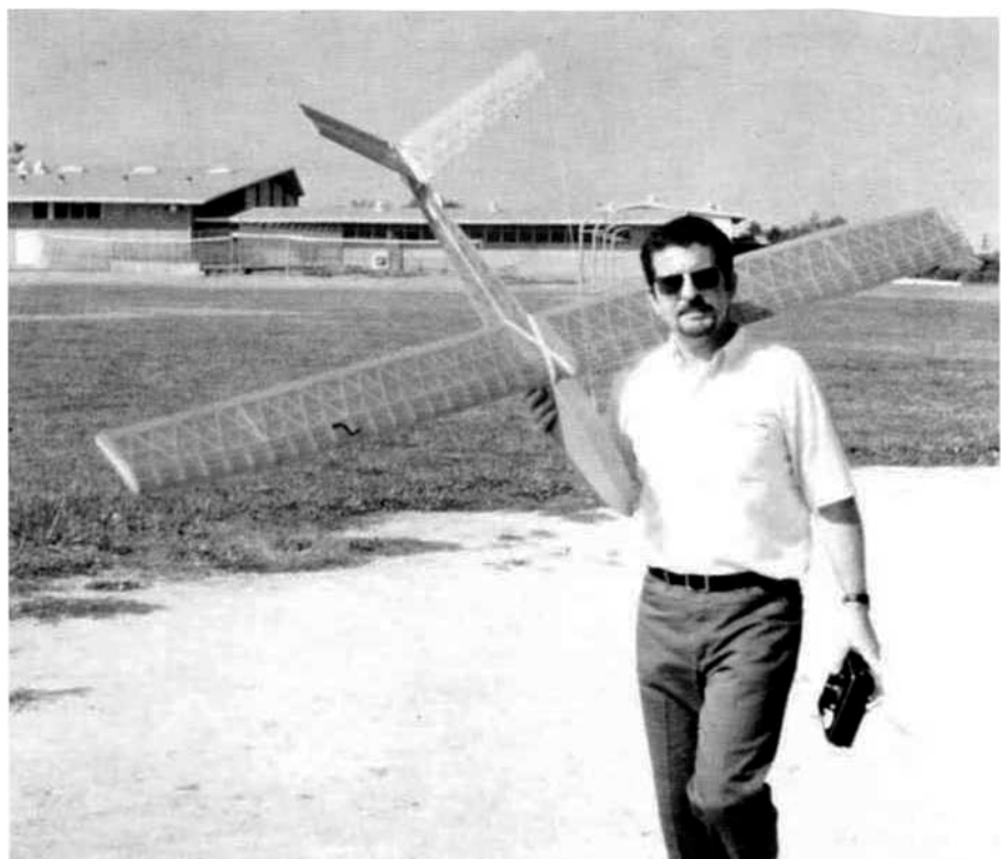
The designer and the plane. Note the strong free flight influence in the construction of the wing and stab. Wing airfoil is HLG type; curved to the high point and then straight to the trailing edge.
