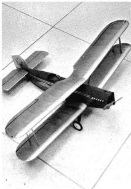
Deviations from scale are increased dihedral and stabilizer area. Makes trimming easier.
