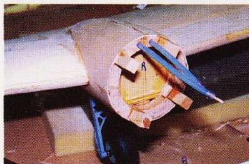
Almost everything happens in the wing. Note the amount of plumbing, for the fuel tanks and the retracts (above left). Robart makes the optional scale retracts (above right) for the model. One nacelle completed (below left), ready for the engine mount. Clean installation of wheel in the well, the cylinder head, and the muffler (below right).
