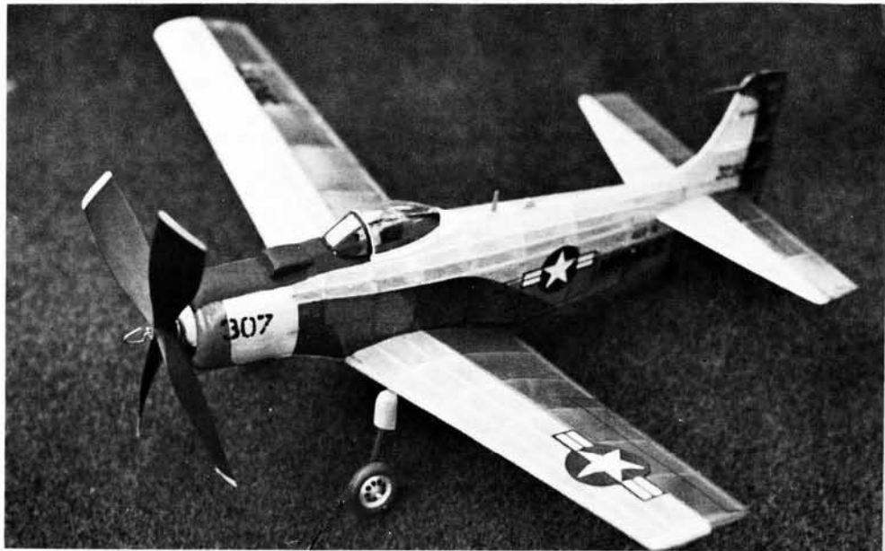
Modeled after a particular aircraft shown in color in the Profile Publication (No. 60), this model stands out in its basic red and white with black trim. Colored tissue used for covering.
