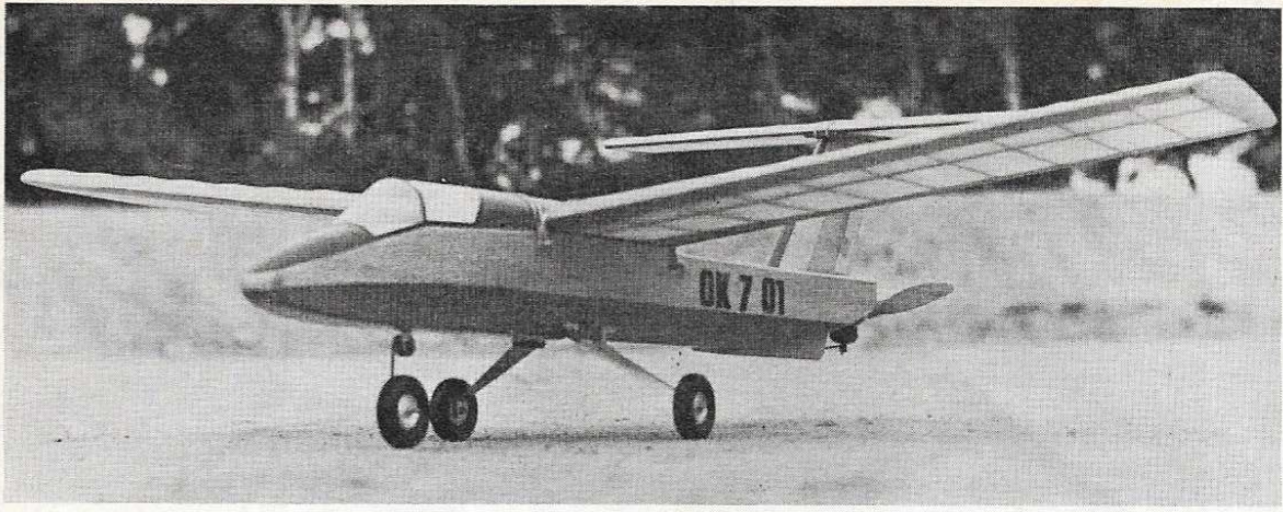
High T-tail and engine-prop at rear, give otherwise-standard simple craft a sleek jet-age look.
