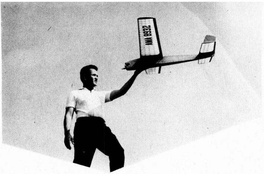
Optional sheet or a built-up stab. Only rudder control is necessary, though install whatever you wish. Design intended to build up fast, get you in air, to practice.
