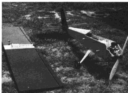
Almost finished, controls installed before gluing down the fuselage top. Note rails around aileron servo for wing alignment.
