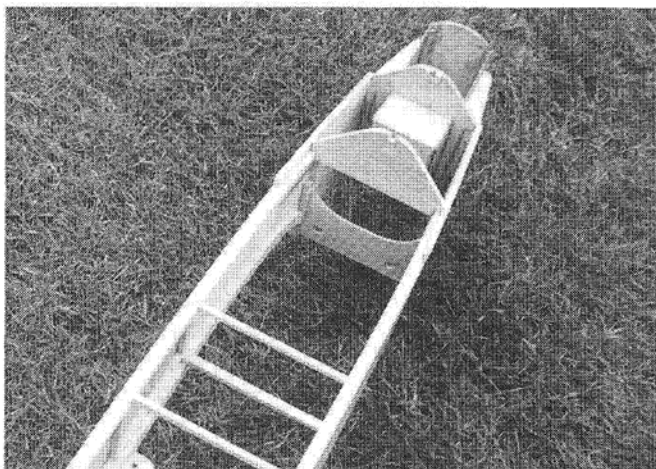
More formers added to fuselage.
