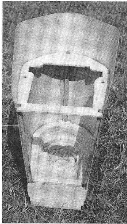
Note keyhole slots for fixing cowl to front former.
