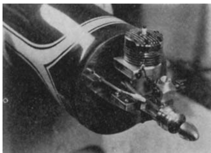
A neat-looking front end. Inside the cowl a beam-mounted Enya .60 TV. Note optional polished-aluminum firewall face.
