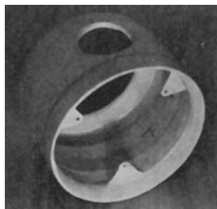
The cowl is made up with cross grained laminations of 1/4 in. balsa. Interior is epoxied.
