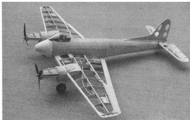
All that's left to do is the sheeting of the tops of the nacelles and the application of covering.
