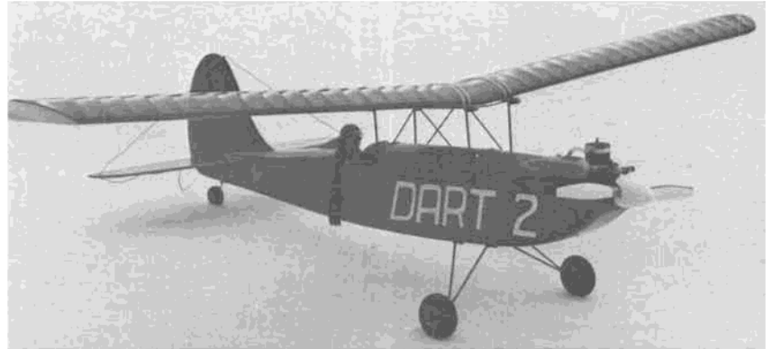
The completed Dart 2 ready for test flights. This one is powered with a Thunder-Tiger .25, but the Dart 2 will fly very nicely on a .19. (That's snow under those tires, not concrete!)
