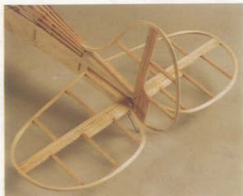
The laminated outlines on the tail group are light and strong. Note the block fill between the fuselage and fin.
