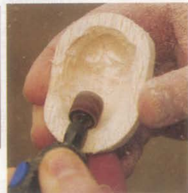
Dremel's new Lithium-Ion cordless rotary tool made quick work of shaping and hollowing the wheel pants, cowl and headrest. I used 150 and 220-grit sandpaper for final smoothing.
