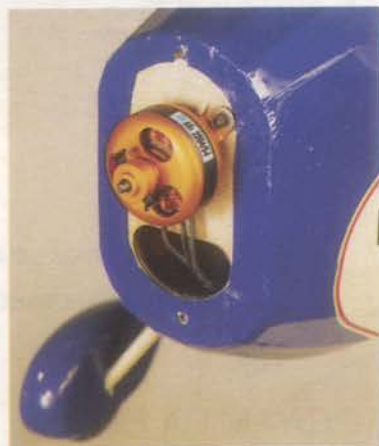
The low profile AXI 2204/54 is easy to mount on the front of the firewall, and provides plenty of silent power for spirited flight.
