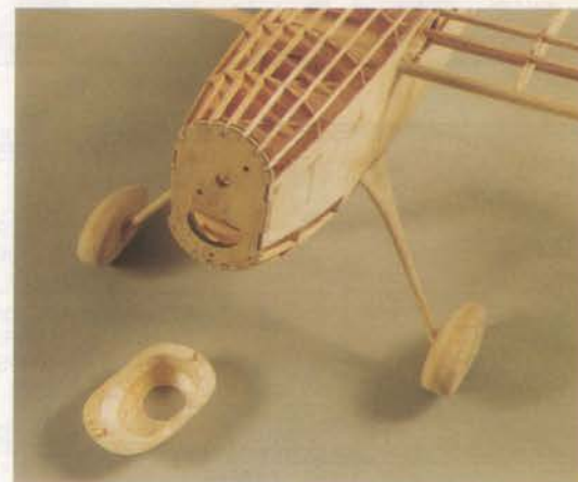
The lightweight structure combines a few unique ideas with traditional stringer and former construction.
