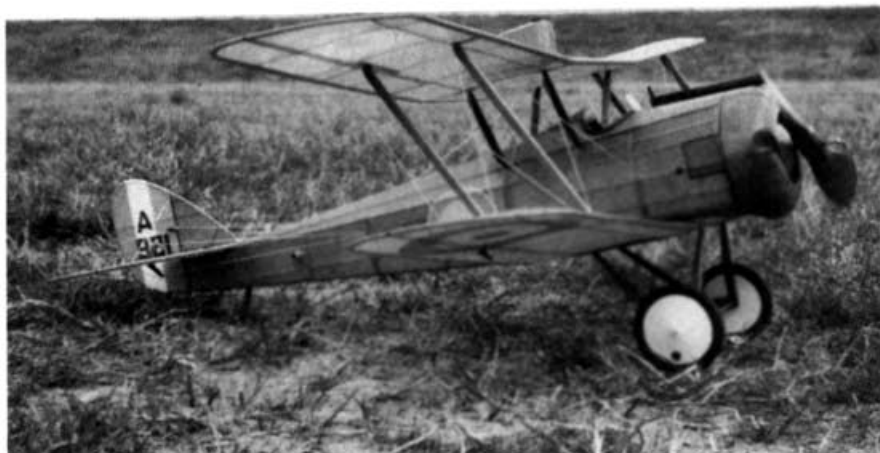
In this quarter profile shot of the D.H. 5 (above), you can easily see its negative stagger, especially in the rear rake of the interplane struts. Note also the fair amount of scale external rigging, for both control surfaces and bracing. This top view (below) shows how the single machine gun is offset to the left.
