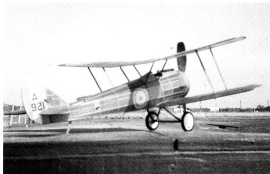
The cross section of the D.H. 5 fuselage is a little unique, starting with the tubby round cowl up front, transitioning, just aft of the cockpit, to a hexagonal shape all the way to the tail.
