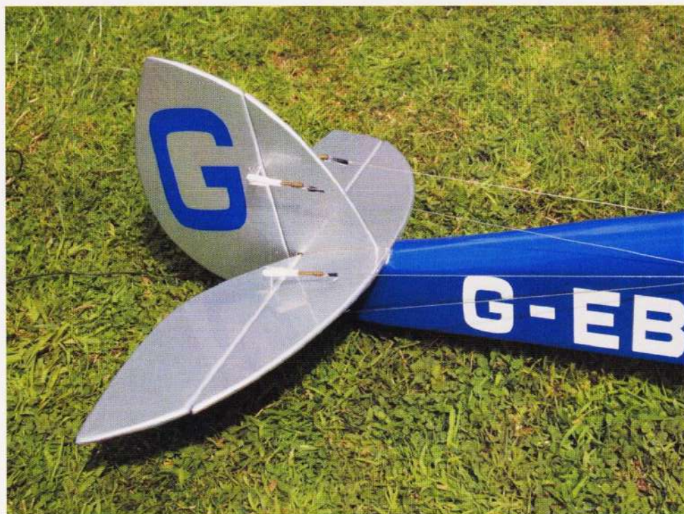
Closed-loop connections to rudder and elevator.
