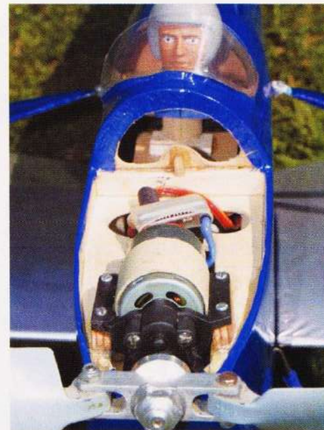
Motor and speed controller installation. Note cut-out in F1A.
