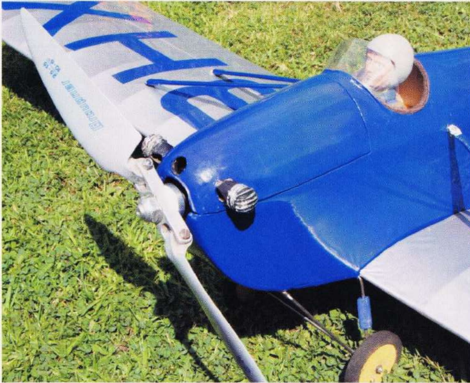
The dummy engine cylinders are attached to the cowl access hatch to complete the original look.
