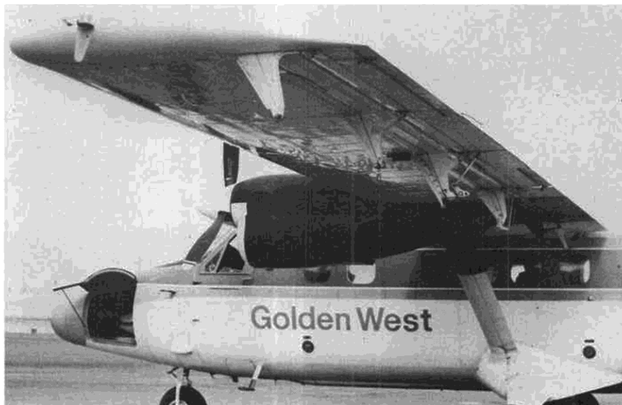
Complicated hinging mechanism provides for a Fowler flap effect on the ailerons, even as they are being used for ailerons. Convenient hatch for baggage . . . or ballast, in a model!
