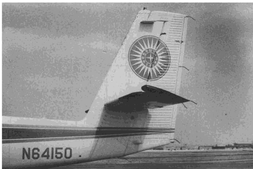
This photo reveals the actual rudder hinge line of the Twin Otter. Note full-length trim tab, and aerodynamic counterbalance at top, also small "stab", possibly to avoid turbulence at tip.
