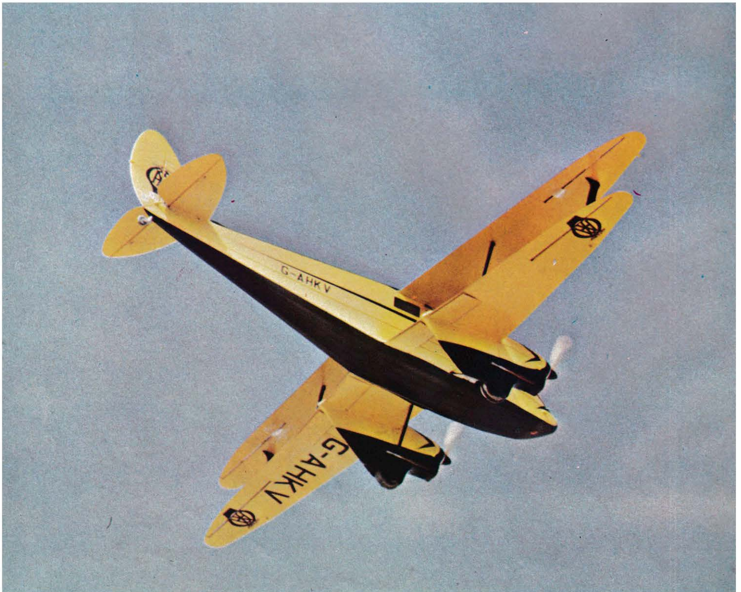
The Rapide has a top wingspan of 96 inches, being 2 inch-to-the-foot scale.
