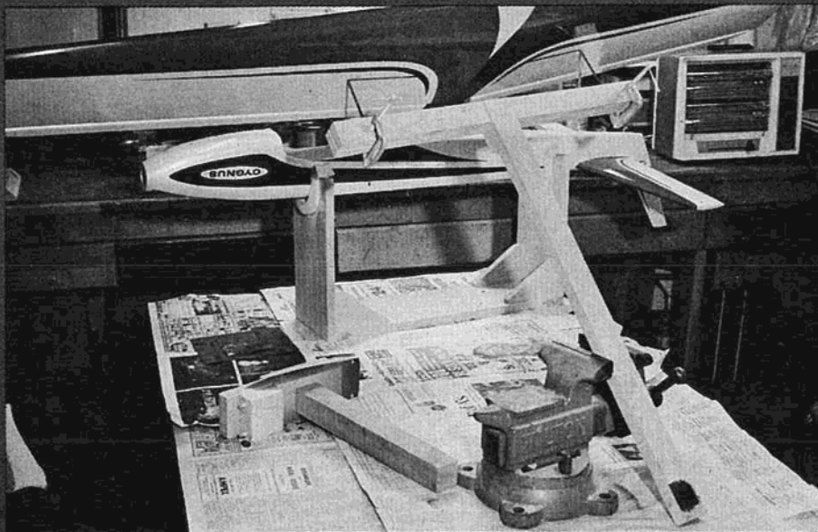
Completely painted fuselage and wing. Jig in foreground.
