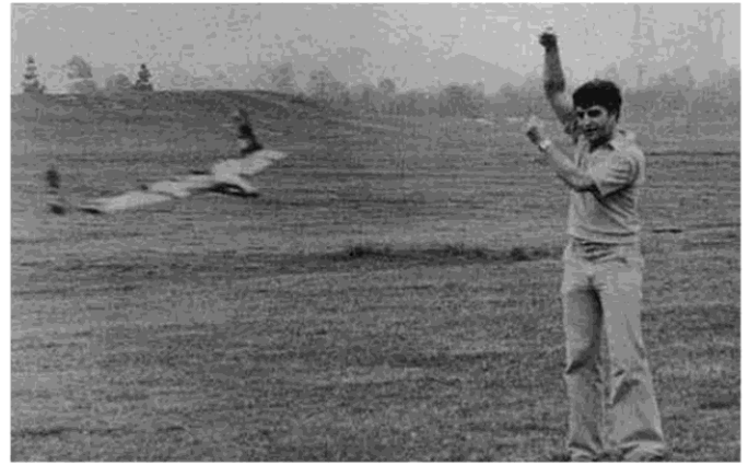
Author-designer, Larry Renger demonstrates the testing technique used for determining CG location and trim settings for maximum stability. Model is swung around right side up and inverted . . . when it flies like this, it's ready to fly R/C.
