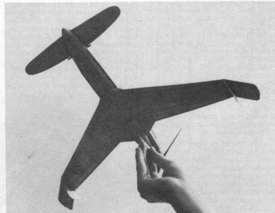
Underside details reveal landing gear doors, belly scoops. Rubber peg is just aft of the knock-off forward surfaces. An interesting R/C scale project possibility, now that Tom has problems solved.
