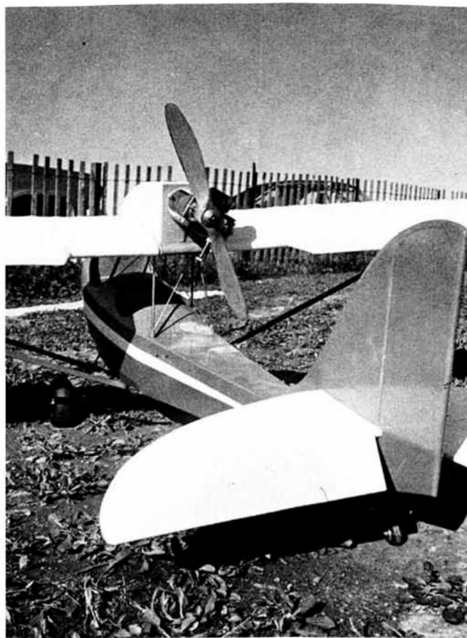
Here's a good view of left-hand prop. You can get left-hand cranks for some engines, but carving a prop isn't bad. It last forever.
